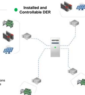
**Virtual Power Plant (VPP)** - A centralized processing server analyzes regional conditions and distributes commands to local DERs to maximize reliability of the local grid. These commands are tailored to the local onsite generation and designed to maximize the utilization of these resources.
